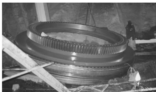
Fig.8 Dismantled TBM ring gear & main bearing
