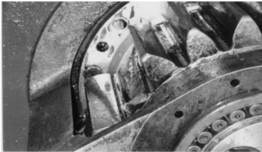
Fig.10 Two broken tooth on pinion
