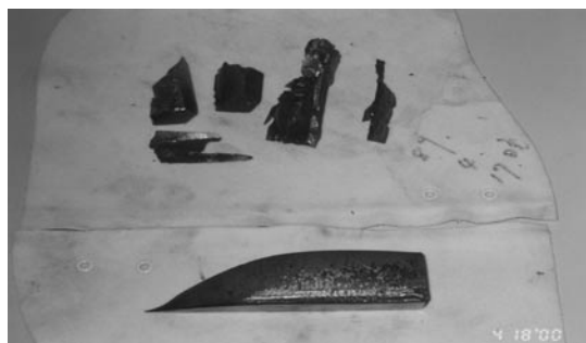
Fig.6 Broken fragments of ring gear & pinion
